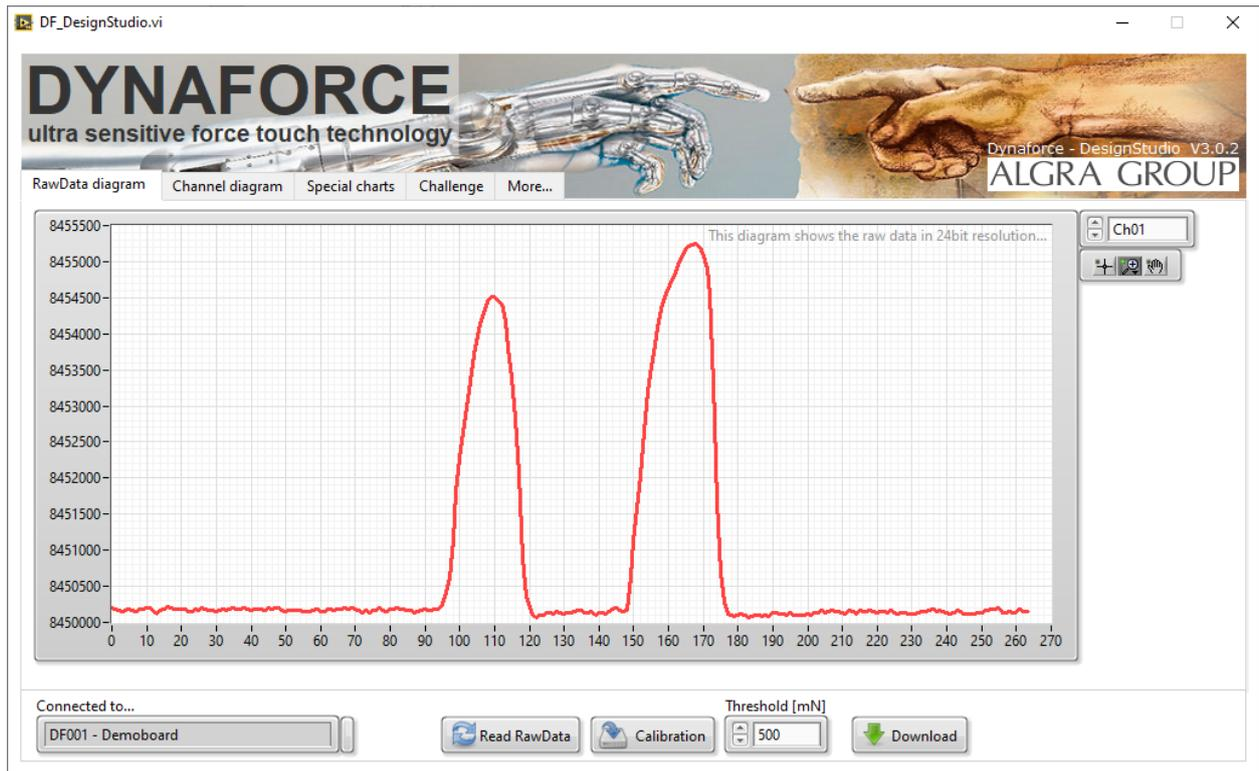
The *RawData diagram* shows the raw data of every key (channel). Each key is displayed in its own chart in auto scaling mode. You can choose the channel by using the list box (Ch00...) in the upper right corner.
