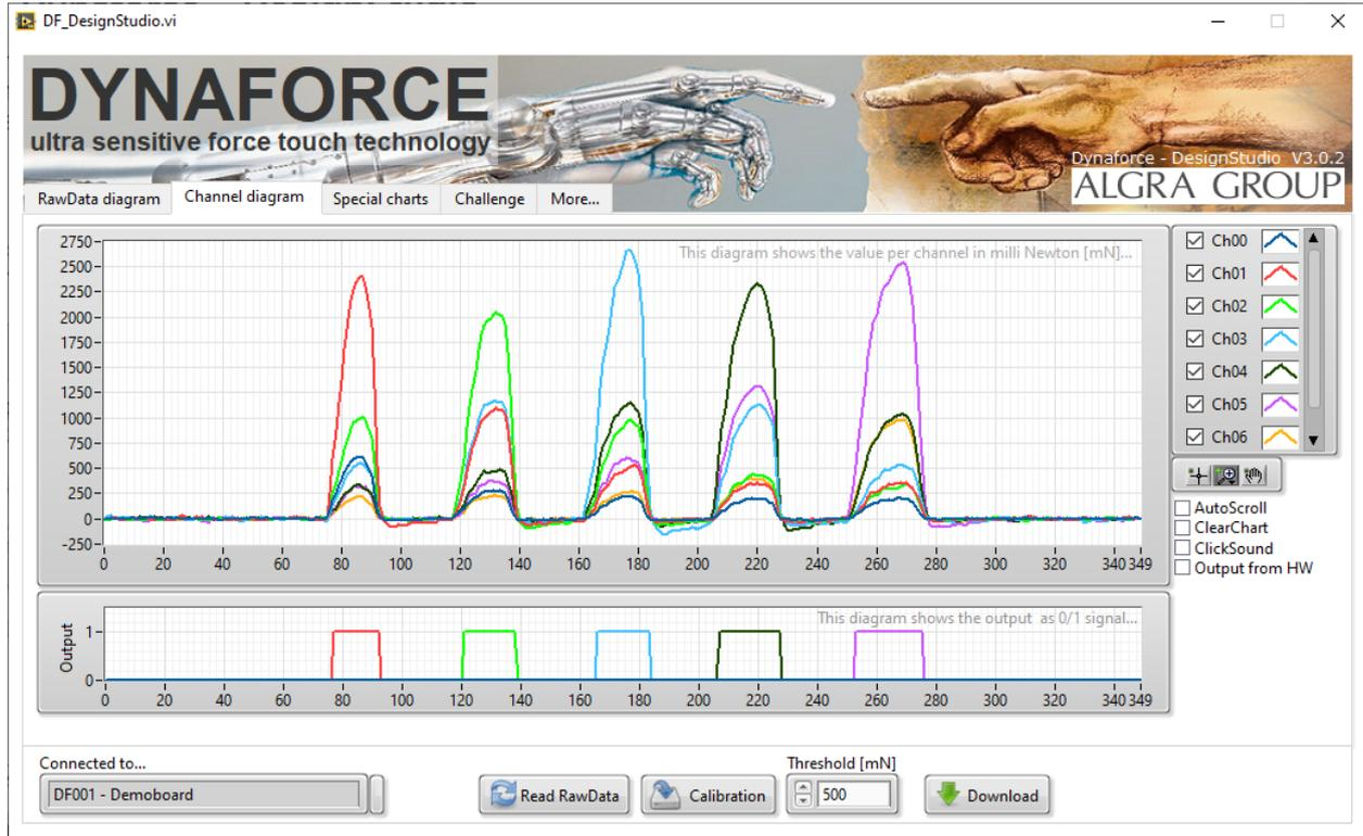
In the *Channel diagram* all channels are displayed in the same graph. The lower diagram shows the output as a binary signal for every channel. In the box on the upper right corner you can select/deselect each channel. With the button *Read RawData* you start/stop the acquisition.
