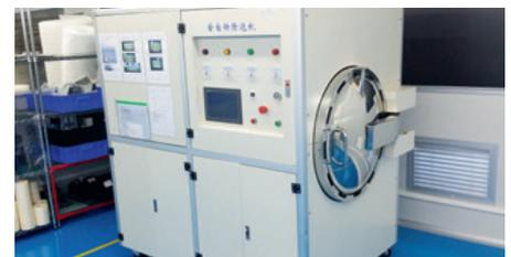
Autoclave for optical bonding
