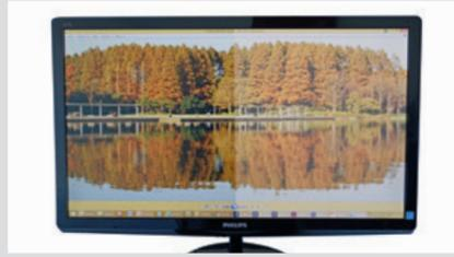
with optical bonding/without optical bonding
